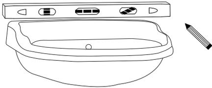
2. Move the sink away from the installation location. For convenience, install the drain and faucet onto the sink before moving on.
