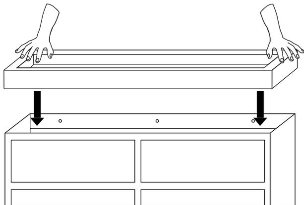
3. Let the assembled vanity sit for 24 hours to allow all the silicone sealant to fully dry. Once dry, proceed to the installation of your faucet and drain.
