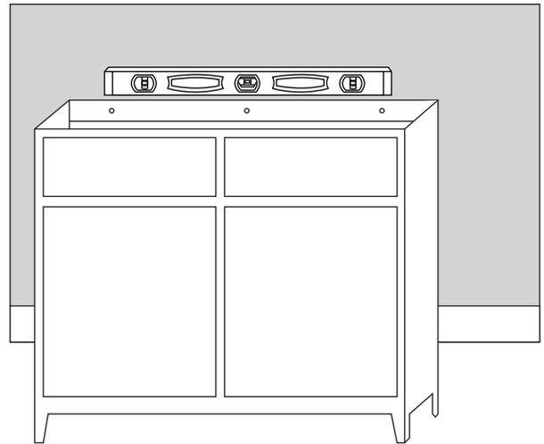
4. Attach the vanity to the wall by screwing through the back of the vanity cabinet. Use the marked stud locations as a guideline. Proceed to step 2 for attaching your sink.
