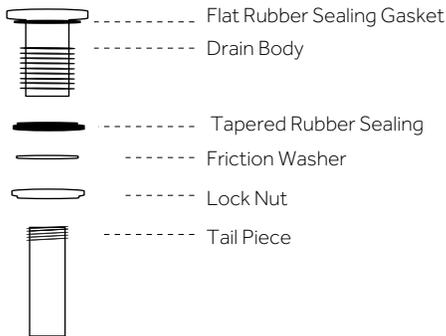
2. Place thread sealant on the threaded section of the tail piece and reattach to the drain body.
